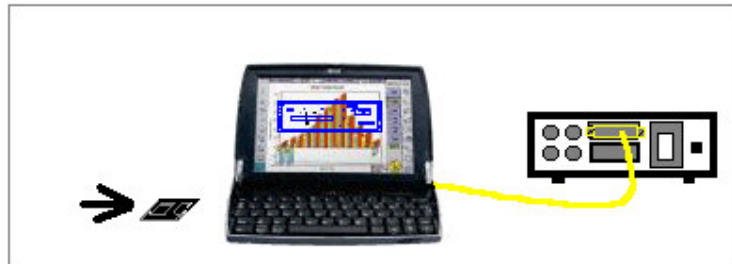
Firmware UPGRADE requires a Floppy disk, Laptop, Serial cable, Smart ping unit
